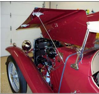
Once the bracket is installed simply raise the bonnet and place the "nut" end of the rod in the bracket and the rubber ball inside the round spring associated with the bonnet latch.
